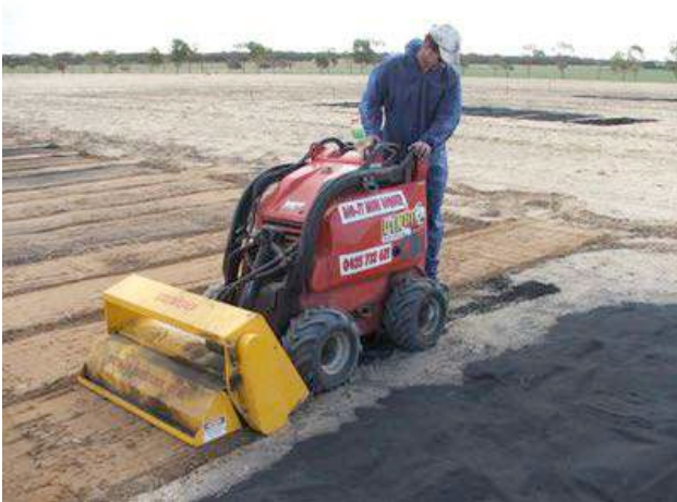
Figure 5. Rotary hoe incorporation of surface spread biochar into the soil at Kalannie.
